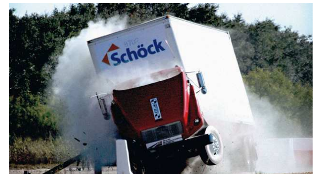
Successful crash test on TL-5/PI-3 barrier wall
